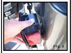
Step 6: Carefully guide the wiring back through the hole and guide the tail light mounting studs into the mounting holes. Install the three lock washers and nuts and tighten evenly, being cautious not to over tighten them. (Fig. 8 & 9)
